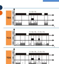
ON for the set interval with STOP (TBS) - on applying the supply voltage U the R relay is in ON position and the set interval T begins. After the interval T has lapsed, the output relay R switches OFF and remains OFF until supply voltage U is interrupted. If the S contact is closed during the interval T, the timer is suspended until the contact is open again.
