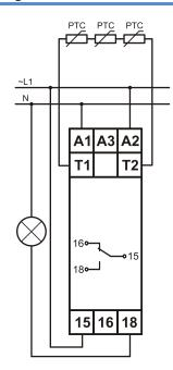
When powering from 230VAC mains, neutral wire N connect to A1 and wire L to A2.
