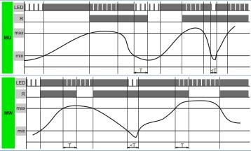
MU (undervoltage) - The output relay R switches into on-position again after the measured voltage exceed the Max-value.
